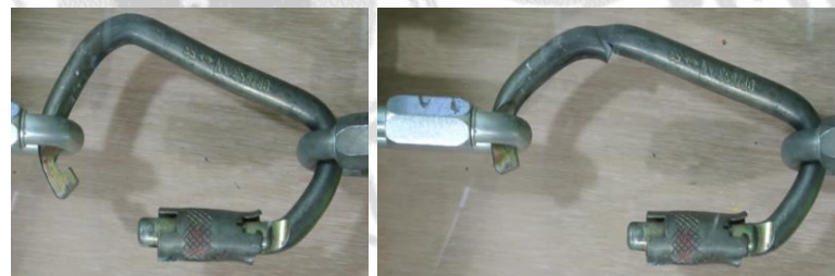
Richard Delaney, RopeLab, 2015. Youtube vídeo: steel carabiner destructive test.
