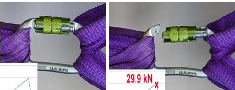
Slacktivity, youtube vídeo: how the shape of a carabiner influences its breaking load
